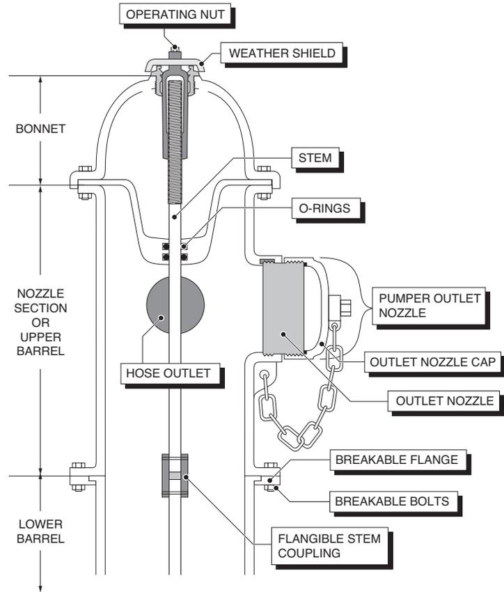
Dry Barrel hydrant with packing stuffing box.
