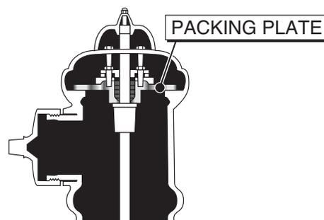
Until very recently, the packing material used in fire hydrants was made from a combination of long fibrous asbestos and graphite. Due to the health hazards in the manufacture of asbestos-based packing, it is no longer available. Fire hydrant manufacturers recommend that existing packing be replaced with
